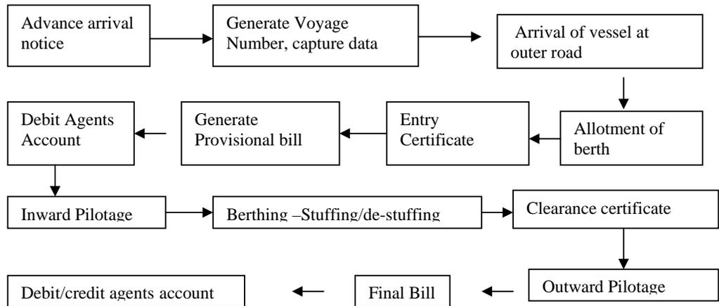
Cargo Information & Billing System covers the billing of cargo related charges such as wharfage, demurrage and equipment hire charges. A flow chart on the cargo billing process is given below:
